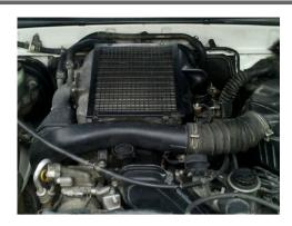
The **Toyota 1KZ-TE** is a 3.0 l (2,982 cc, 181.97 cu-in) four cylinders, four-stroke cycle water-cooled turbocharged internal combustion diesel engine, manufactured by the Toyota Motor Corporation. The 1KZ-TE engine has a cast iron block with 96.0 mm (3.78 in) cylinder bores and a 103.0 mm (4.06 in) piston stroke for a capacity of 3.0 l. Compression ratio rating is 21.2:1.
